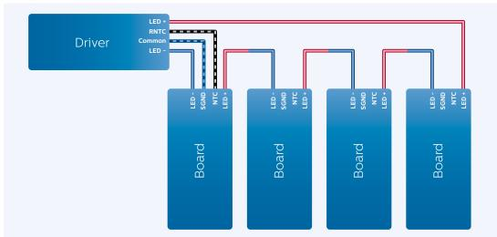
If a system consists of multiple FastFlex boards connected to a single driver:
