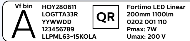
Example label on LED Linear module indicating bin A.
