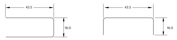
Mounting in cut-out in sheet metal (thickness 0.7 mm to 1.2 mm)
