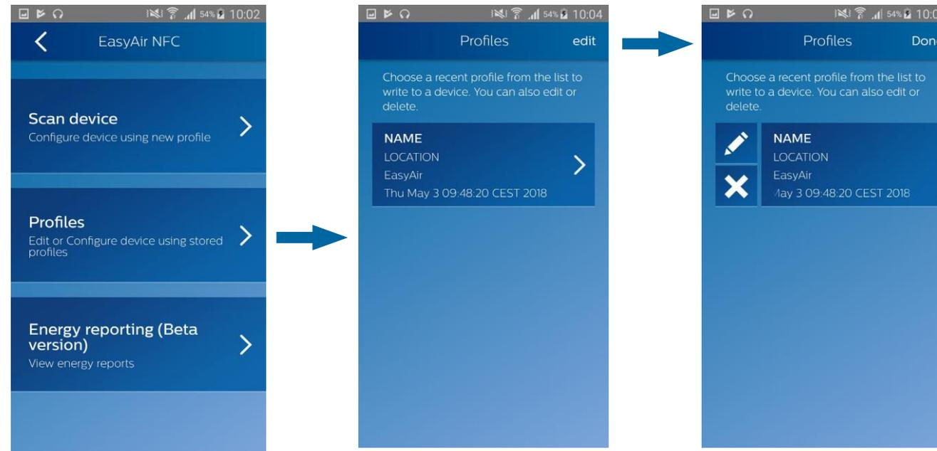
With the NFC App, the user can write back a profile to a single EasyAir sensor.
