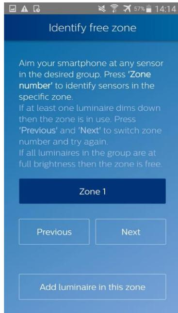
3. Select the zone the luminaire will be added to. In our case, the zones 1 and 2 are used already. Press **Next** to switch to Zone 3.
