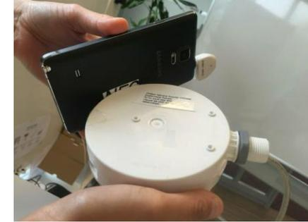
**Note:** Make sure that the NFC reader location is known on the smartphone used. Place the back of the smartphone (where the NFC reader locates) onto the sensor NFC antenna (almost touching) to enable NFC communication.
