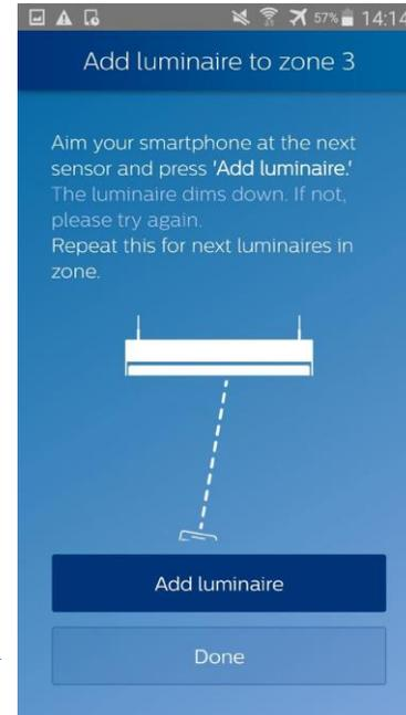
5. Aim the smartphone at luminaire 5, and press **Add luminaire**. If needed, repeat with other luminaires you want to add the new Zone 3. Then, press **Done**.
