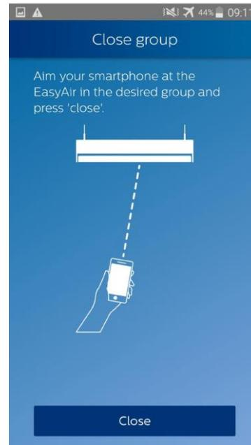
7. Aim the smartphone to the sensor of any luminaire of the group and press **Close**
