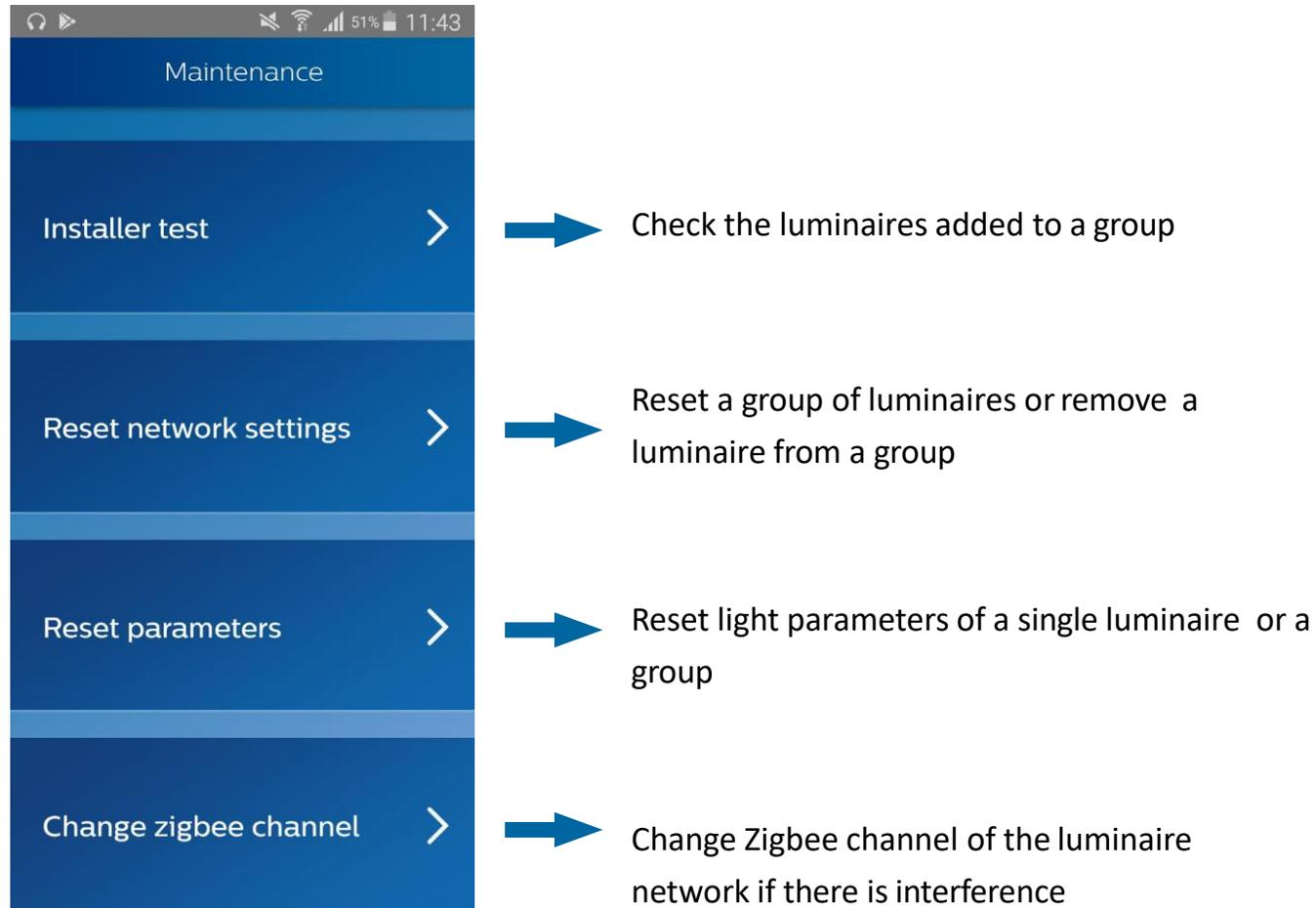
The image shows a mobile application interface for a 'Maintenance' menu. The menu is displayed on a dark blue background with white text. The status bar at the top shows the time as 11:43 and battery at 51%. The menu items are: 'Installer test', 'Reset network settings', 'Reset parameters', and 'Change zigbee channel'. Each item has a white chevron icon to its right. Blue arrows point from each menu item to a corresponding text description on the right side of the image.
