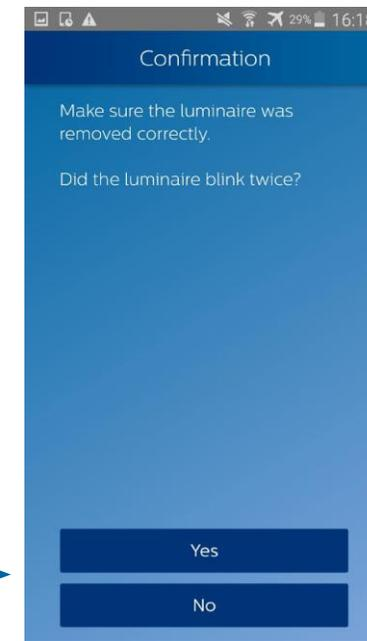
3. Check that the remaining luminaires of the group (luminaire 1) blinked twice
