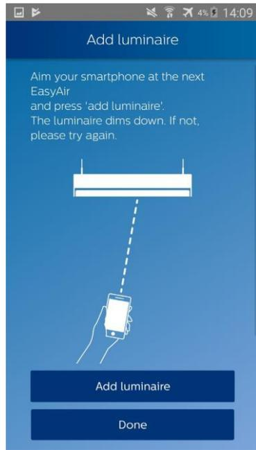
5. Aim the smartphone at the sensor of the luminaire to add in the group, and press **Add luminaire**.
