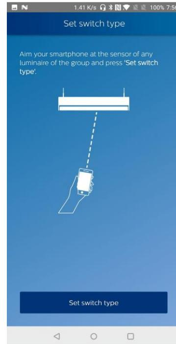
5. Aim the smartphone at any luminaire of the group and press **Set switch type**
