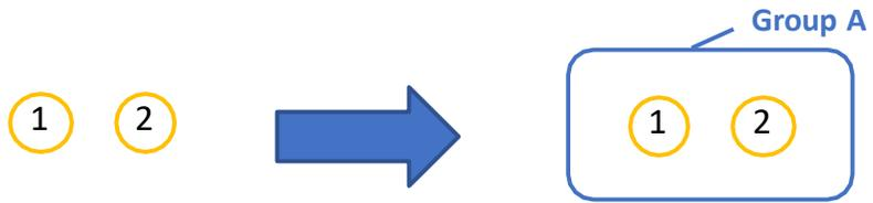
**Note:** For proper group functioning it is recommended to limit the number of luminaires (sensors) in a group to 40.
