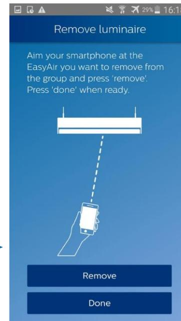
2. Aim the smartphone at the sensor of the luminaire you want to remove (luminaire 2) and press **Remove**. Once ready, press **Done**.
