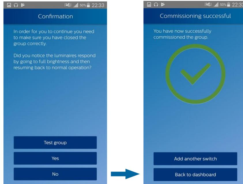
8. Check that the luminaires of the group went to full brightness before resuming to normal operation, indicating the group is closed
