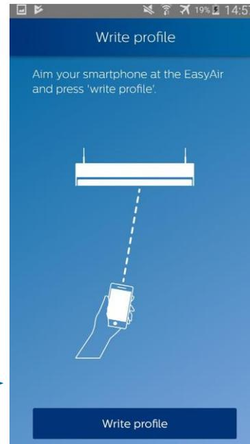
4. Aim the smartphone at the luminaire's sensor, and press **Write profile**
