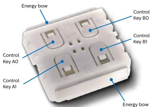
Figure 1 - Outer appearance of Legrand EnOcean module
