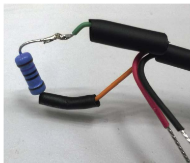
Example of resistor being integrated in the cable
