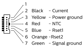
JST connector (driver side) pin layout
