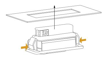
Press springs inwards on both sides before the bracket can slide-in the luminaire hole.
