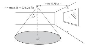
Motion field of view can be reduced using the plastic shield on top of the lens
