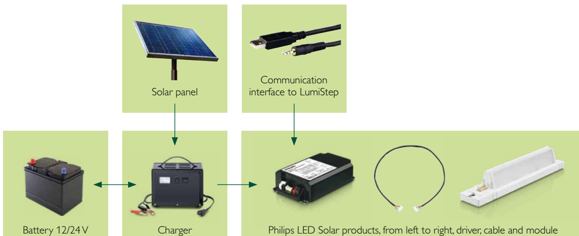
Schematic diagram of a solar-powered system, including Philips Fortimo LED LLM Gen 3 and Xitanium driver
