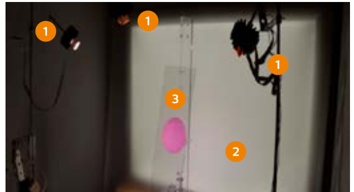
Figure 2: Inside of box. 1 = 3 RGBY LEDs, 2 = background panel (CCT = 3400 K), 3 = meat between glass plates
